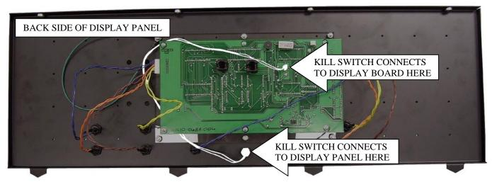
Older display boards will appear slightly different, but the magnetic kill switch will connect in the same locations. The magnetic kill switch in this picture has been made white for better visibility.
